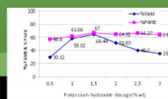
Figure 4 Influence of catalyst dosage during alkaline transesterification on % FAME and % Yield
